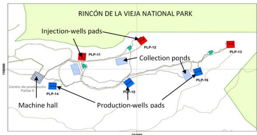
Scheme of the Las Pailas II power plant. Injection-well pads (PLP-11, 12 & 13) have only three injection wells each. (Credit: ICE. Taken from the source.)
