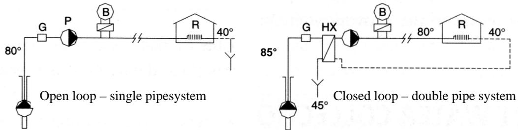
Figure 10. Two main types of district heating systems. G=gas separator, P=pump, B=boiler, R=radiation heating, HX=heat exchanger (Dickson and Fanelli, 2003).
