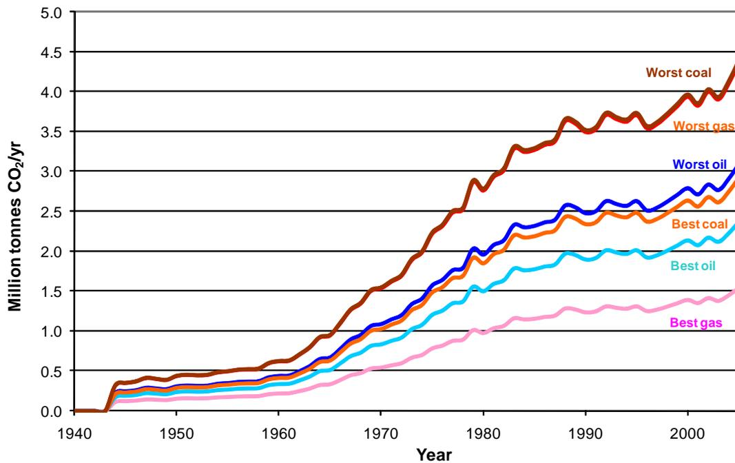
Figure 15. CO<sub>2</sub> savings using geothermal water in Reykjavik (Iceland) compared to other energy sources 1940-2006. Total avoidance 90 million to 110 million tonnes of CO<sub>2</sub> emissions depending on the type of fossil fuel(s) replaced by geothermal resources (Gunnlaugsson, personal communication 2008).
