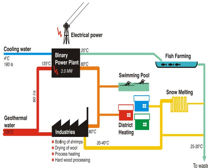
Figure 8. An idealized diagram showing cascaded uses of geothermal energy.
