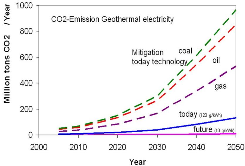
Figure 21. Mitigation potential of geothermal power plants in the world based on data of Table 6 and assumptions for emission of 120 g CO<sub>2</sub>/ kWh for today and 10 g CO<sub>2</sub>/ kWh for future technology.
