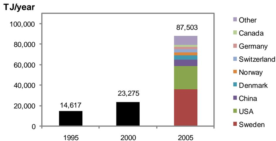
Figure 13. Worldwide growth of ground source heat pump applications and the leading GHP countries. Data from Lund et al. (2005).
