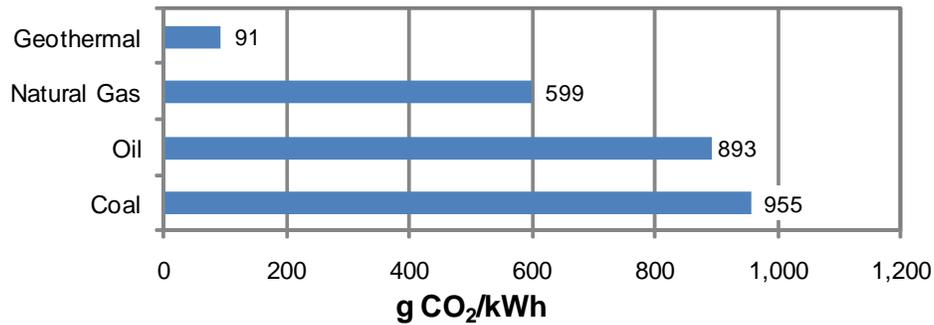
Figure 14. Comparison of CO<sub>2</sub> emission from electricity generation from different energy sources in the USA. Data from Bloomfield et al. (2003).
