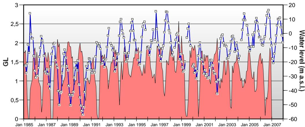
Figure 22. Production in Gigaliters (in red) from the Reykir low-temperature field and the water level (black line with data points) in well MG-28 (observation well) from 1985 to 2007 (Ivarsson, 2007).
