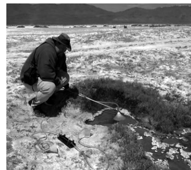
Arizona State geochemist Matthijs van Soest samples surface water in the northern Basin and Range. The sample is collected without direct exposure to air and stored in the copper tube, foreground left, which will be sealed by crimping.
