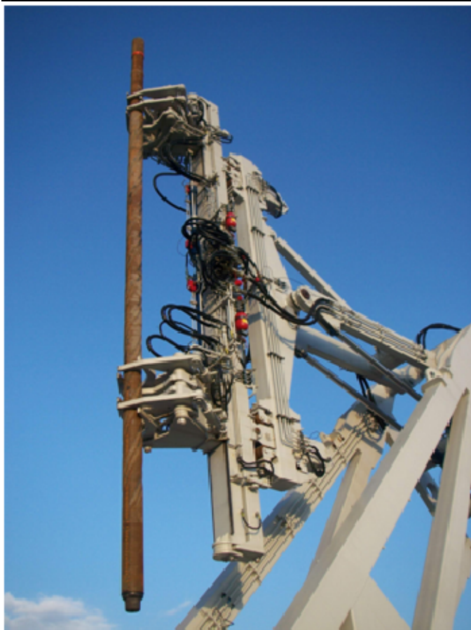
Figure 2: The automatic pipe handling system increases safety at work and reduces the number of staff required.
