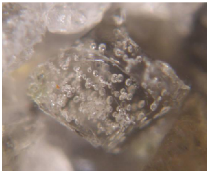
Colorless rhyolitic glass shard (approx. 1 mm across) with spherical vesicles. Photo from the IDDP website, www.iddp.is
