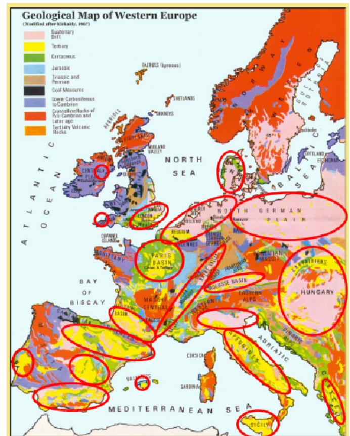
This map shows geological basins in Europe which are possible for cost-effective geothermal electricity projects ; future developments might allow other regions to be used too. There is also current potential in Romania, Bulgaria and Greece, which are not covered on the map (base map Kirkaldy, 1967).
