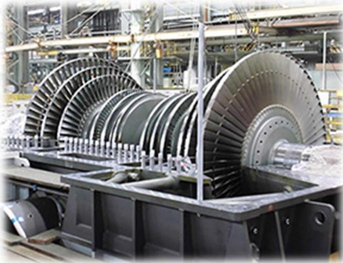
*Steam turbine for geothermal power plant (Photo: courtesy of MHPS, Ltd.).*
